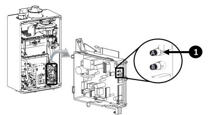
2. Use the  $\blacktriangle$  (Up) and  $\nabla$  (Down) button on the controller to select a setting number (See Parameter Settings Table).
