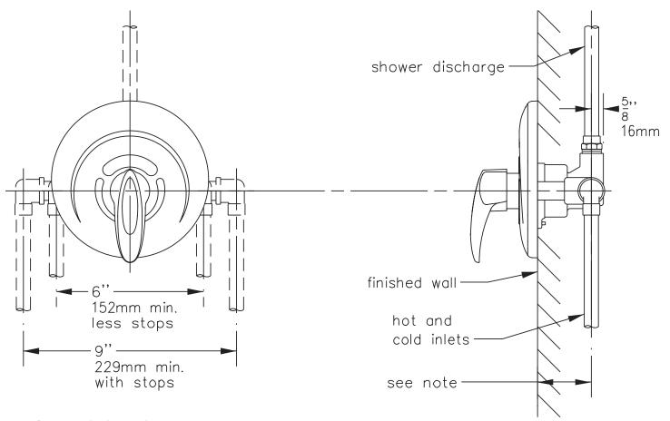
NOTE: 2-3/8" (60mm) min. 3" (76mm) max. 2-5/16" (59mm) fixed dim. metal stall. Valve inlets and outlets are 1/2" (13mm) IPS connections.
