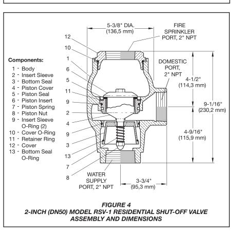
As indicated above, domestic system usage can reduce the pressure available to the fire sprinkler system. However, when utilizing the Model RSV-1 Valve, you do not need to include additional hydraulic flow of the domestic system, when otherwise required by NFPA standards (NFPA 13R), to determine the minimum possible residual (flowing) pressure available to the fire sprinkler system.
