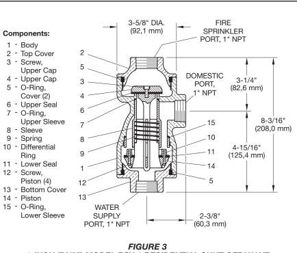
1-INCH (DN25) MODEL RSV-1 RESIDENTIAL SHUT-OFF VALVE ASSEMBLY AND DIMENSIONS
