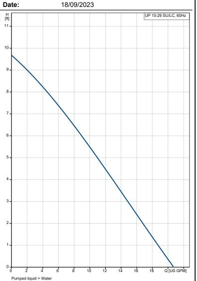
Liquid temperature during operation = 140 °F Density = 61.35 lb/ft³
