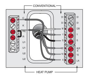
Fig. 312. Inserting wires in thermostat terminal block.
