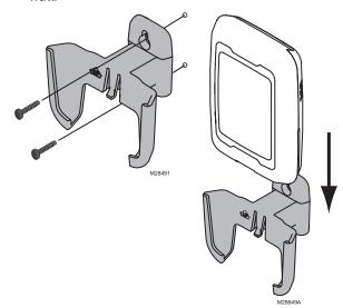
Fig. 72. Mounting Outdoor Sensor.
