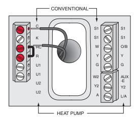
Fig. 20. Inserting wires in thermostat terminal block.
