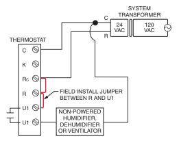
Fig. 330. Wiring a non-powered humidifier, dehumidifier, or ventilator.
