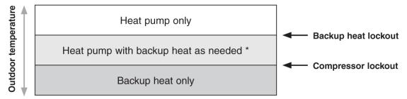
No backup heat unless indoor temperature drops to selected Backup Heat Droop setting, or Backup Heat Upstage Timer expires. **Heat pump stays ON when backup heat turns on.**
