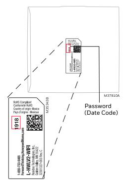
Fig. 4. Finding thermostat password.
