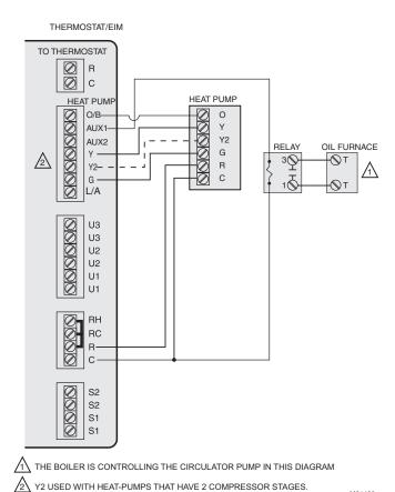
Fig. 320. Heat pump with oil forced air backup.
