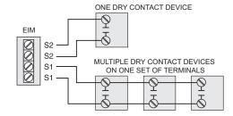
Fig. 157. Wiring dry contact devices.
