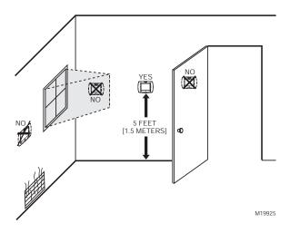
Fig. 14. Selecting thermostat location.
