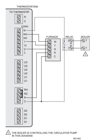
Fig. 323. Hot water radiant heat with backup heat (single zone application).
