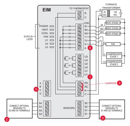
Fig. 314. EIM wiring guide - conventional systems.
