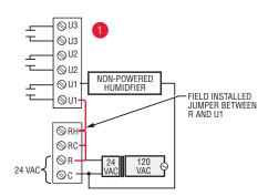
Fig. 335. Typical hookup of non-powered humidifier.
