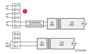
Fig. 333. Typical hookup of powered ventilation.
