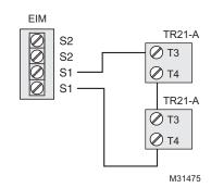
Fig. 349. Wiring 2 TR21-A sensors.
