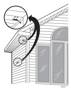
Fig. 73. Typical locations for C7089U1006 Outdoor Sensor.
