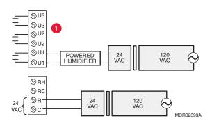
Fig. 332. Typical hookup of powered humidifier.
