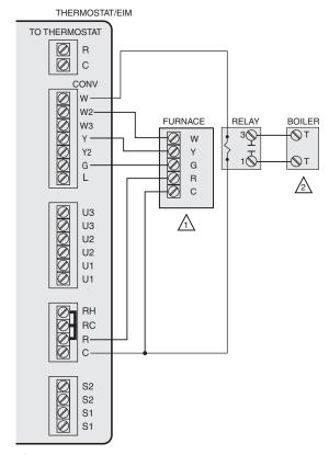
CONFIGURE THE THERMOSTAT TO ENERGIZE THE FAN WITH A CALL FOR HEAT.
