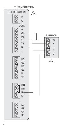
CONFIGURE THE THERMOSTAT TO ENERGIZE THE FAN WITH A CALL FOR HEAT.
