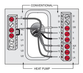
Fig. 19. Thermostat wired directly to equipment.
