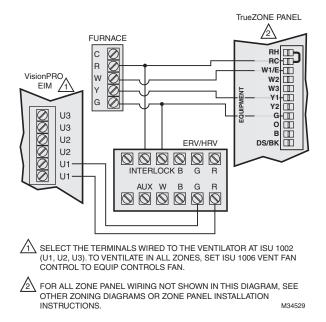
Fig. 352. RedLINK 2.0 VisionPRO thermostat with an HZ432 zone panel and a ventilator.
