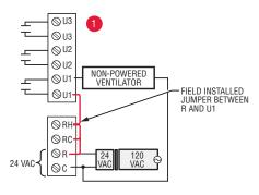
Fig. 336. Typical hookup of non-powered ventilation.
