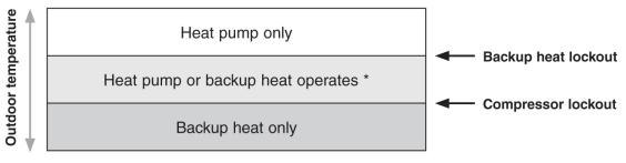
No backup heat unless indoor temperature drops to selected Backup Heat Droop setting, or Backup Heat Upstage Timer expires. **Heat pump turns OFF when backup heat turns on.**
