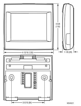
Fig. 1. Dimensions of thermostat in in. (mm).
