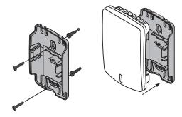
Fig. 74. Mounting Indoor Sensor.
