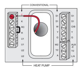
Fig. 18. Connecting C wire to terminal block.
