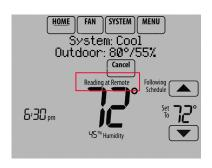
Fig. 303. Reading temperature at the Portable Comfort Control.
