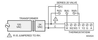
Fig. 318. Series 20 hot water heat.
