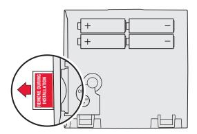
Fig. 21. Remove coin cell battery tab.
