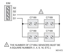
Fig. 346. Wiring 4 C7189U sensors.
