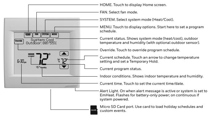
Fig. 79. Quick reference to commercial display.
