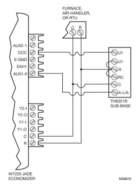
Fig. 339. Economizer control with economizer fault alert using TH8321R without EIM.
