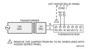
Fig. 319. AQ2000 series panels or other hot water relay panels.
