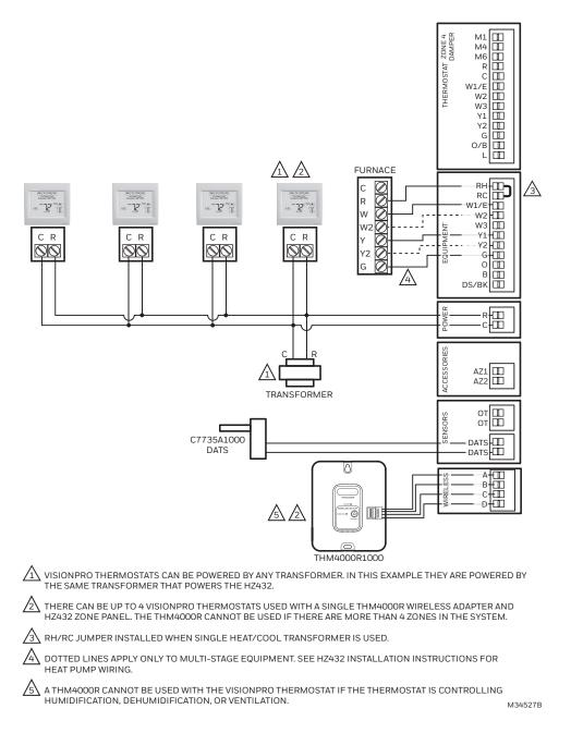
Fig. 350. RedLINK 2.0 VisionPRO thermostats with an HZ432 zone panel and no IAQ control.
