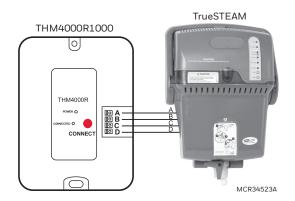
Fig. 50. Connect button on TrueSTEAM wireless adapter.
