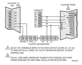
Fig. 353. RedLINK 2.0 VisionPRO thermostat with an HZ432 zone panel and a TrueDRY dehumidifier.
