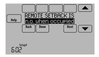
4. Select a Remote Setback Time Delay. The Remote Setback Time Delay forces the thermostat to wait before it switches from occupied settings to the Remote Setback settings. When set to 0 minutes, the thermostat will switch from occupied settings to the Remote Setback settings immediately when the room is unoccupied.
