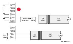
Fig. 334. Typical hookup of powered dehumidifier (whole house dehumidifer).
