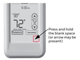
Fig. 48. Restarting the linking process.
