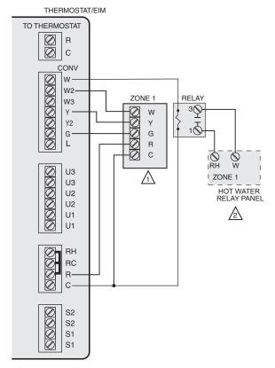
HZ311, HZ322, OR HZ432 ZONE PANELS COULD BE USED TO CONTROL A FORCED AIR FURNACE ZONED WITH DAMPERS.
