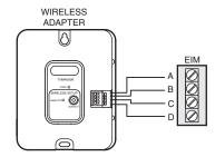
Fig. 6. THM4000R1000 Wireless Adapter wired to the EIM.
