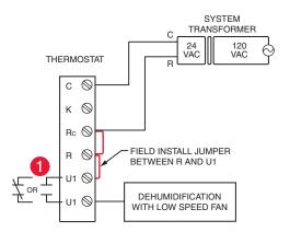
Fig. 329. Dehumidification with low speed fan using a variable speed blower.
