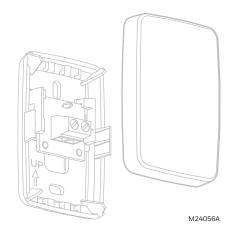
Fig. 75. Remove the cover.
