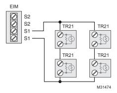
Fig. 348. Wiring 4 TR21 sensors.
