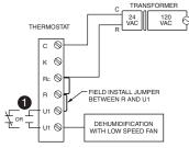
Wire the thermostat U1 terminal to the low speed fan for dehumidification control at the equipment as shown. The relay can be set to normally open or normally closed in the installer setup.
