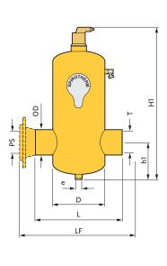
All Spirovents fabricated and stamped in accordance with ASME Section VIII, Division 1 for unfired pressure vessels.
