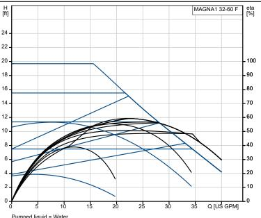
Pumped liquid = Water Liquid temperature during operation = 140  $^{\circ}$ F Density = 61.35 lb/ft³
