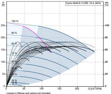
Losses in fittings and valves not included Pumped liquid = Water Liquid temperature during operation = 68 °F Density = 62.29 lb/ft³
