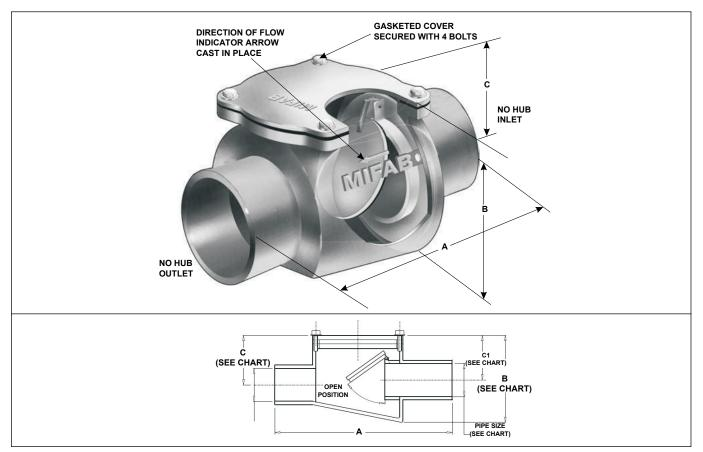
Note: Do not use for pressurized applications; for gravity flow only. Backflow protection is prevented when the valve is obstructed by debris or sludge; clean regularly.
