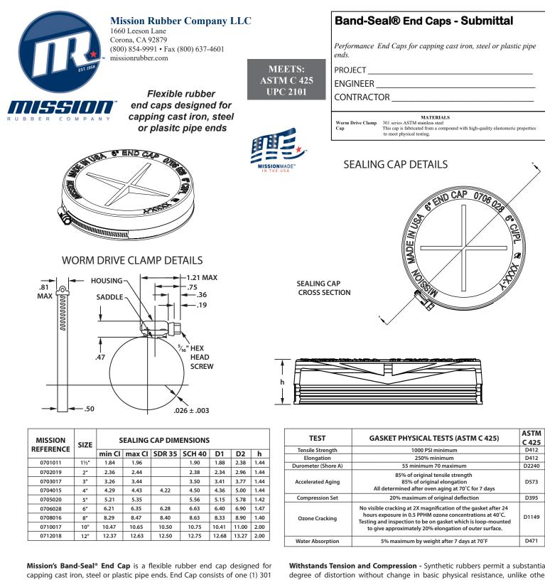
**Mission's Band-Seal® End Cap** is a flexible rubber end cap designed for capping cast iron, steel or plastic pipe ends. End Cap consists of one (1) 301 series stainless steel worm drive clamp, over a molded one-piece elastomeric sealing cap. Available in sizes 1½" to 12".
