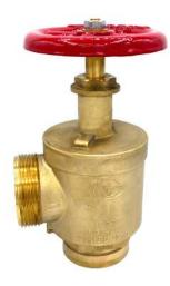
Heavy Duty 2-1/2" (65 mm) brass, 300 lbs (2070 KPa) pressure tested approved angle hose valve. Lightweight cast brass body, Forgeline Bonnett and Seat Assembly. UL/ULC listed and FM Approved. Specify regional hose thread for outlet.
