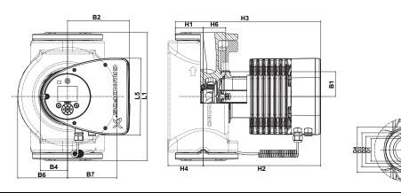
Dimensions in. [mm] Pump type L1 L5 В1 B2 В4 В6 В7 D1 D2 4.37 [111] 1.57 [40] 1.93 [49] MAGNA3 40-180 F (N) D4 D5 Н1 H2 НЗ Н4 Н6 2.4 [61] 3.15 [80] 0.5 [12.8] 11.97 [304] 2.76 [70] 1.97 [50]
