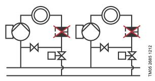
Fig. 9 Reduced need for a pump throttling valve
