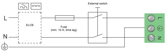
Fig. 36 Example of typical connection, 1 x 230 V  $\pm$  10 %, 50/60 Hz
