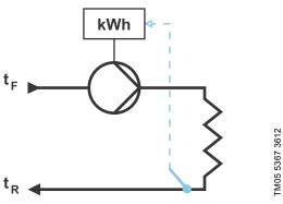
Fig. 28 MAGNA3 with built-in heat energy meter
