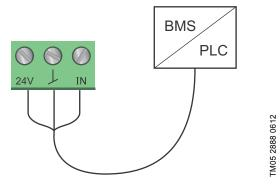
Fig. 43 Example of external signal for the control via BMS or PLC
