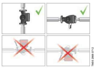
Fig. 35 Installation positions
