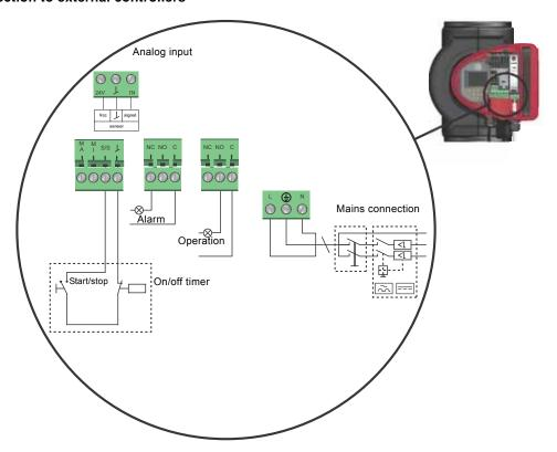
Fig. 37 Example of connections in the control box
