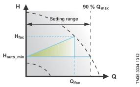
Fig. 10 FLOW<sub>ADAPT</sub> control
