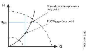
Fig. 21 Constant-pressure control with FLOW LIMIT
