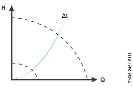
Fig. 16 Differential-temperature control
