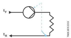
Fig. 15 Pump with external sensor
