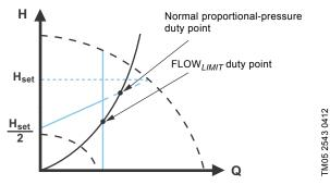
Fig. 20 Proportional-pressure control with  $FLOW_{LIMIT}$
