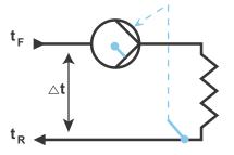
Fig. 17 Pump with external sensor
