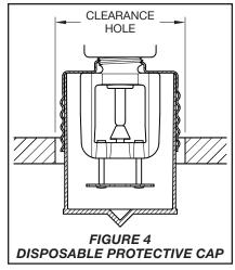
**Step 5.** Replace the Protective Cap by pushing it upwards until it bottoms out against the Support Cup. (Refer to Figure 4.) The Protective Cap helps prevent damage to the Deflector and Arms during ceiling installation and/or finish. You can also use the Protective Cap to locate the center of the clearance hole by gently pushing the ceiling material up against the center point of the Protective Cap.
