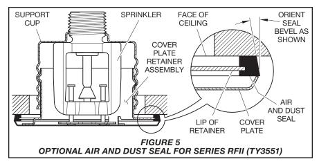
Care must be exercised to avoid damage to the sprinklers - before, during, and after installation. Sprinklers damaged by dropping, striking, wrench twist/slippage, or the like, must be replaced. Also, replace any sprinkler that has a cracked bulb or that has lost liquid from its bulb. (Ref. Installation Section.)
