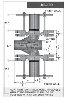
\*MC-10 is tested to support a 500 lb. load with the rear anchor support.
