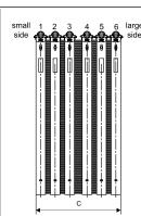
Size 12": Tighten bands alternatively to minimum 60-inch pounds torque in the following sequence: 3,2,1 - 4,5,6.
