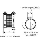
Sizes 2"- 4": Tighten bands alternately to minimum 60-inch pounds torque, in the following sequence:1-2.
