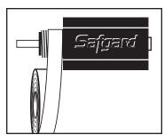
Apply Teflon® tape to the threads of the Model 1100M. Do not use pipe dope or other pipe sealants.
