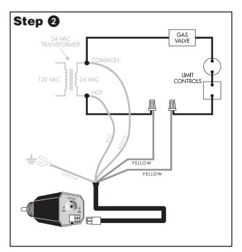
Cut-off the connectors and strip the ends of the two yellow wires of the Model 1100M harness. Break into the burner circuit between the *hot* side of the transformer (R) and other limit controls. Connect either YELLOW wire to the *hot* side. Connect the other YELLOW wire in series with other limit controls. **Important:** The switch contacts of the low water cutoff (yellow wires) must be wired in series with all other limit and operating controls (as shown above).
