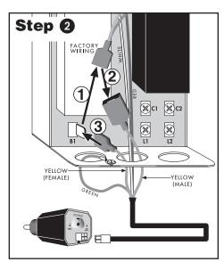
① Unplug the factory-wired quick connect from terminal **B1** and ② plug into YELLOW wire with *male* connector. ③ Plug YELLOW wire with *female* connector into terminal **B1**.
