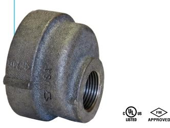
Anvil standard and extra heavy cast iron threaded fittings are manufactured in accordance with ASME-B16.4 (except plugs and bushings, ASME B16.14). Dimensions also conform to Federal Specifications, WW-P-501 (except plugs and bushings WW-P-471).
