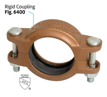
The Figure 6400 Rigid Coupling is specially designed to provide a rigid pipe connection to meet the specific demands of copper tubing installation size 2"-8". Fast and easy swing-over installation of the rugged lightweight housing produces a secure rigid pipe joint. Available with Grade "EP" Copper EPDM flush gap style gasket. Gasket has service temperature range of -40°F to +250°F.
