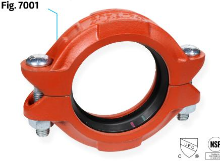
The Gruvlok Fig. 7001 Coupling forms a flexible grooved end pipe joint connection with the versatility for a wide range of applications. Services include mechanical and plumbing, process piping, mining and oil field piping, and many others. The coupling design supplies optimum strength for working pressures to 1000 PSl (69 bar) without excessive casting weight.
