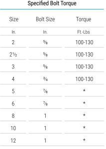
\* Torque required to bring housing metal-to-metal contact.
