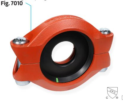
The Fig. 7010 Reducing Coupling makes it possible to directly connect two different pipe sizes, eliminating the need for two couplings and a reducing fitting. The specially designed reducing coupling gasket with a center rib assures proper positioning of the gasket and prevents the smaller pipe from telescoping into the larger during assembly. Fig. 7010 Reducing Coupling allows for working pressure ratings up to 500 PSI (34.5 bar). Not recommended for vacuum applications.
