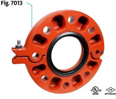
The Gruvlok Fig. 7013 300# Flange allows direct connection of Class 250 or Class 300 flanged components to a Gruvlok piping system. The two halves of the 2" thru 12" sizes of both Gruvlok Flanges are drawn together by a latch bolt which eases assembly on the pipe. A specially designed gasket provides a leak–tight seal on both the pipe and the mating flange face.
