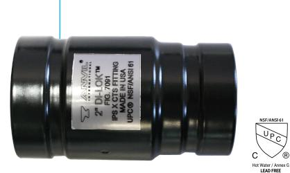
The Gruvlok Fig. 7091 DI-LOK Fitting prevents the formation of a galvanic cell between grooved end steel pipe and copper tube. The separation of copper from steel by the fitting virtually eliminates the galvanic cell created by the dissimilar metals.
