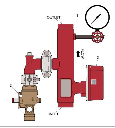
MODEL RM-1 COMMERCIAL RISER MANIFOLD 1-1/2 THROUGH 6 INCH (DN40 - DN150)
