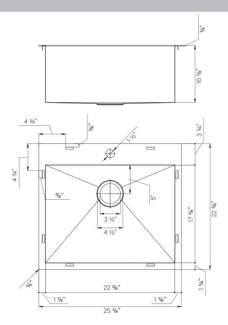
**ATTENTION!** Dimensions may vary by up to 3/8". It is highly recommended to pull all dimensions of actual model for installation and measuring purposes.
