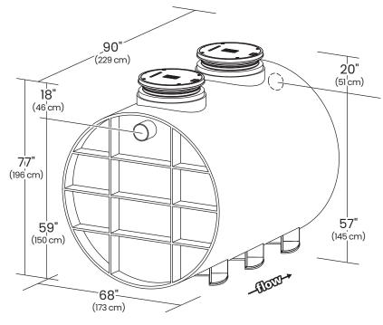
This unit is certified to ASME A112.14.3 (Type C) and CSA B481.1 and includes an
