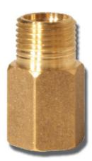
Designed to be used as sprinkler head extensions when a drop nipple length has been cut too short or when the finished ceiling has changed from its intended location. Using the appropriate length extension will allow for realignment of the sprinkler head without removing and recutting the drop nipple.
