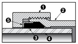
(1) Threaded end-nuts screw onto the threaded body
