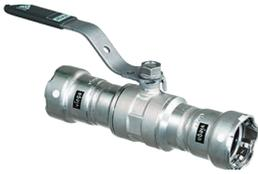
The MegaPress 316 stainless steel ball valve is equipped with a full port, 316 stainless steel 2-piece body and stainless steel press ends. The ball valve features an EPDM sealing element, a 420 stainless grip ring, a 304 stainless separator ring, EPDM stem seals, a locking stainless steel handle, and Viega's Smart Connect® technology for easy identification of unpressed connections during pressure testing.
