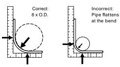
NOTE: Tubing may be bent to a minimum of 5  $\times$  O.D. with approved bend support.
