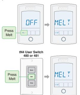
Once manually started, the snow melting system continues to operate until the time set by the Manual Melt Run Time setting in the Set Temp menu elapses.
