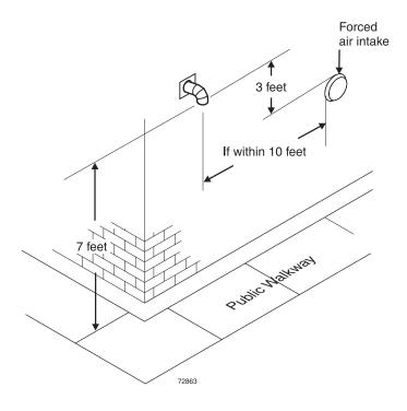
Figure 5 Maintain minimum clearances from doors, windows and snow line
