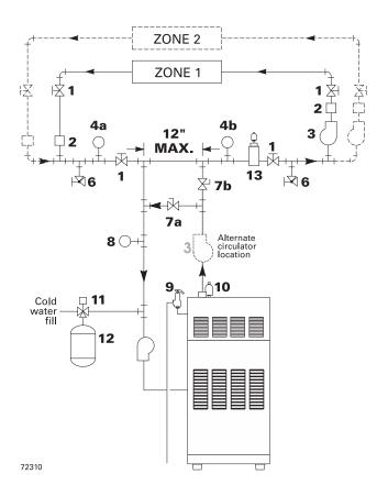
Figure 17 Primary/secondary piping Zoning with zone valves
