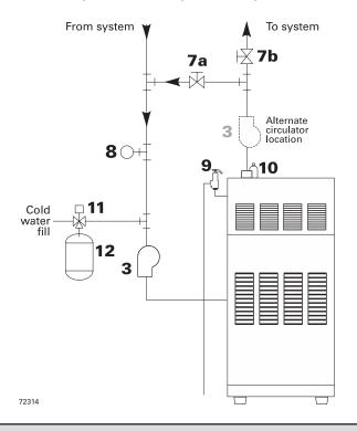
System-bypass piping as shown in Figure 20 can be used with either zone valve or circulator zoning. When used with circulator zoning however, the boiler circulator (item 3), must be piped as shown. It cannot be used as one of the zoning circulators.
