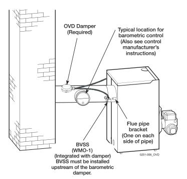
Figure 4 Top outlet breeching connection for OSB-3 through 6 with OVD damper.
