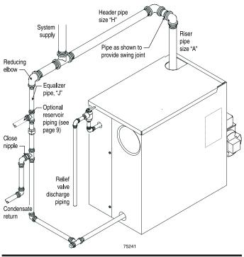
Figure 9 Recommended piping, OSB-6, piping for parallel-flow systems only
