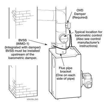
7. OVD Vent damper kit Part Number 381-800-515WT must be installed in all installations. The vent damper is supplied with the boiler. Refer to the damper instruction manual and to Figures 3 and 4 for damper location. A blocked vent shutoff switch (BVSS) is integrated into the damper wiring harness.
