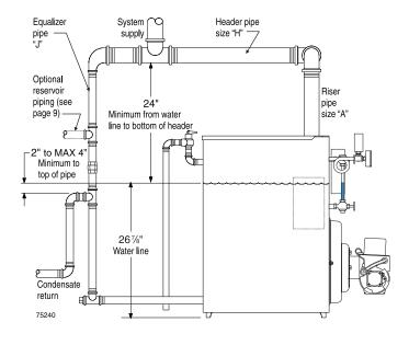
Figure 8 Recommended piping, OSB-6, piping for parallel-flow systems only
