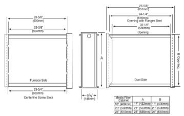
NOTE: Media cabinet is matched to the bottom opening on furnace. May also be used for side return
