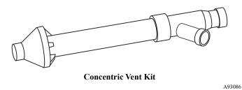
A concentric vent kit allows vent and combustion-air pipes to terminate through a single exit in a roof or side wall. One pipe runs inside the other allowing venting through the inner pipe and combustion air to be drawn in through the outer pipe.
