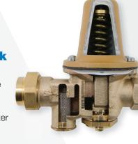
valve body. This action is controlled by an adjustable spring-loaded diaphragm and disc. Even if the supply water pressure fluctuates, the WPRV ensures a constant flow of water at a functional pressure as long as the supply pressure does not drop below the valve's set pressure. Watts WPRVs are adjustable and typically preset at 50psi.
