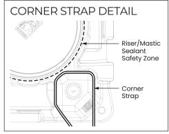
**NOTE:** Ensure that tie-down strap does not touch riser or mastic or tank to riser seal will be compromised
