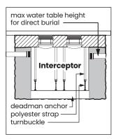
high water table scenarios must be installed with an anti-flotation anchor kit. Models GB-50, GB-75, and GB-250 use model AK1 anchor kit. Model GB-500 uses model AK2 anchor kit for use with deadmen anchors. Models GB-1000, GGI-750 and GGI-1500 use model AK3 anchor kit for use with deadmen anchors.
