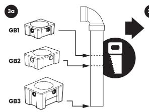
Trim internal vertical piping assembly at premarked location.
