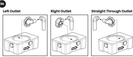
Dry fit pumpout adapter and vertical pipe assembly as shown for chosen port location (Left, Right or Straight Through). Hand tighten into place. Ensure that vertical piping assembly is pointed down (as shown) and ensure that there is at least  $1/2^{"}$  of clearance between the vertical pipe and floor of unit. Remove internal piping assembly for cementing.
