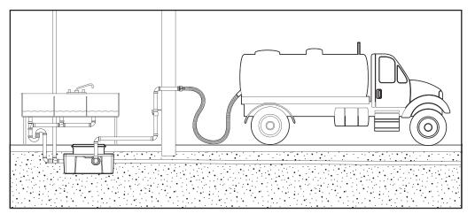
Run Sinks to ensure interceptor is full of water. Attach pumper hose to 3" cam and groove fitting. Turn on pump, make sure interceptor is pumped out and inspect pumpout plumbing for leaks.
