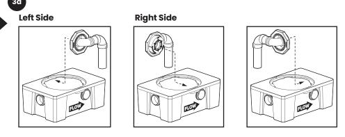
Place internal pipe assembly as shown for chosen port location (Left, Right or Straight Through). Securely hand tighten pumpout adapter retaining nut.
