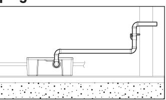
Install 3" or 2" PVC piping, connections, valves and/or hardware from the interceptor pumpout port to pumpout hook-up location (Not included with this kit). Maximum quantity of 6 elbow fittings. Max. height from static water line of interceptor to hook-up is 21 feet. Max horizontal distance from interceptor to pumper truck (including hose) is 100 feet.
