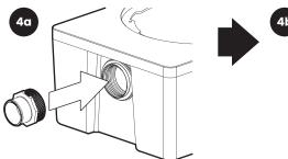
Install the supplied 3" plain end fitting at the pumpout port using pipe thread sealant or tape.
