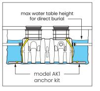
areas, floodplains and areas that receive storm water. Great Basin™ and Billy Goat™ models that are direct buried in high water table scenarios must be installed with an anchor kit.
