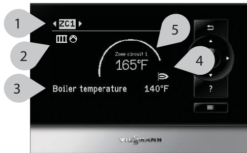
ZC Fixed Setpoint Configured
